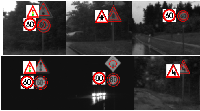
Figure 5: Traffic sign detection (and recognition)
