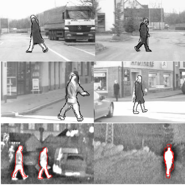
Figure 7: Pedestrian detection results
