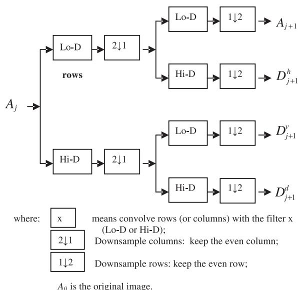
Figure 2 Decomposition of an image,  $A_j$  into a coarser approximation sub-image,  $A_{j+1}$ , and detail sub-images  $D_{j+1}^h$ ,  $D_{j+1}^v$  and  $D_{j+1}^d$ .
