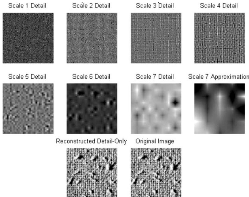
**Figure 9** The reconstructed scale 1–7 detail sub-images, the scale 7 approximation image, the reconstructed detail-only image using wavelet *coif1* and the original WoolMark SM 50 plain degree 1 standard pilling test image.
