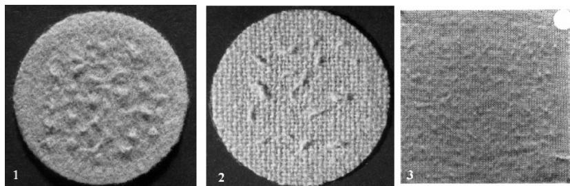
Figure 1 WoolMark® standard pilling test images from (1) SM 50 blanket set; (2) SM 50 plain set; (3) SM 54 lambswool set.
