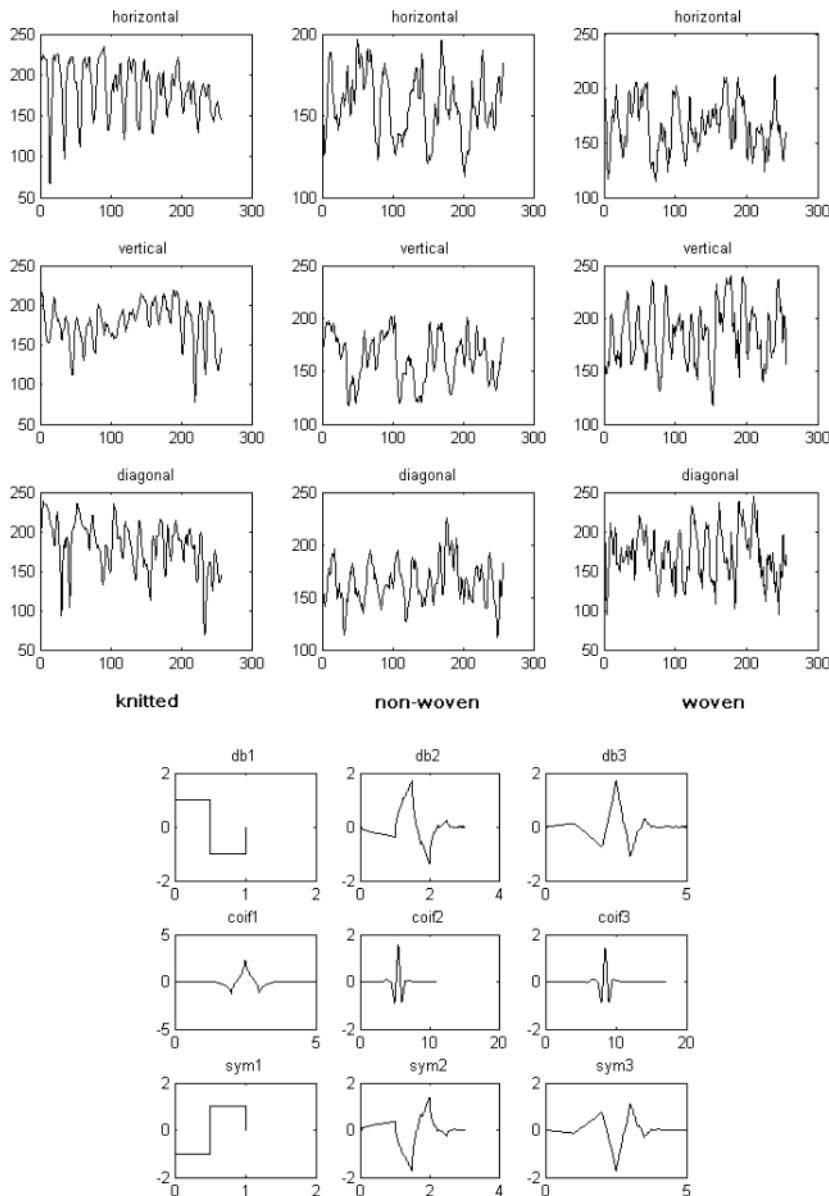
**Figure 3** Typical shapes of data and analysis wavelets.
