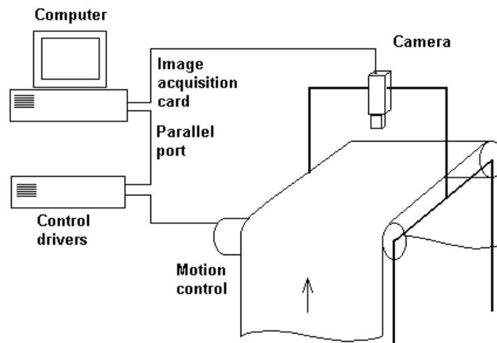
Figure 1. The vision system schematic
