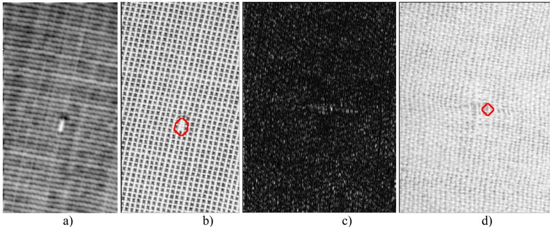
Figure 4. a) and b) results of original images filtered by optimal Gabor filter; c) and d) defect detection after thresholding and region growing
